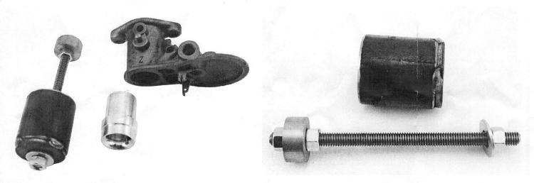
Remove throttle plate and shaft from carburetor. Place shaft through carburetor from flange side. Place cup over shaft. Install nut and tighten until venturi is removed into cup.
